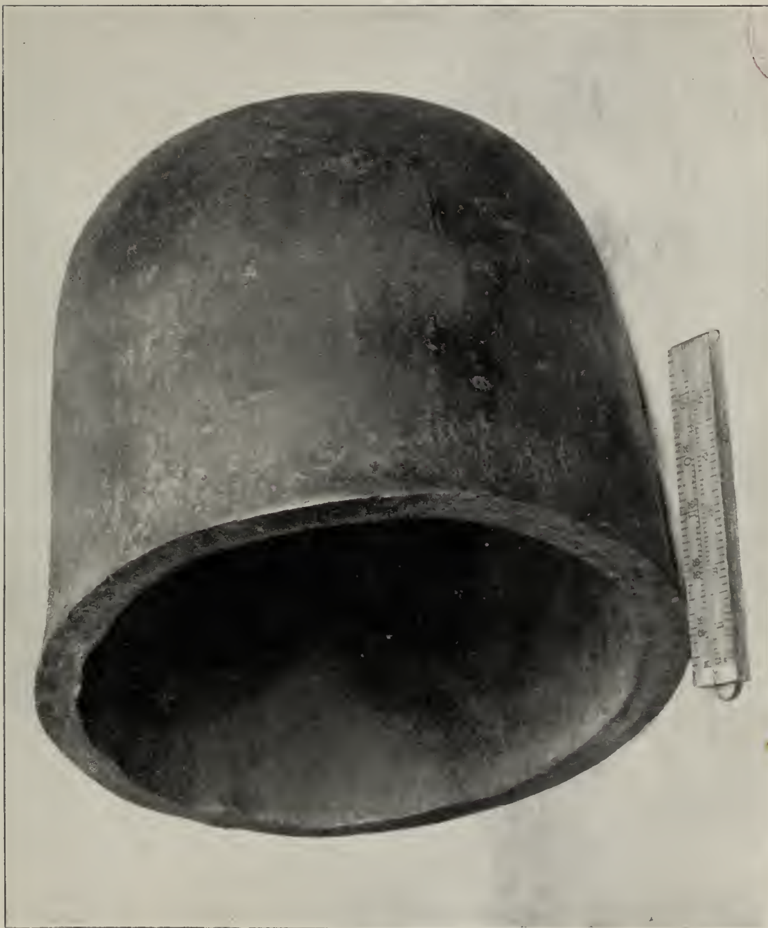
FIG. 56. BESEMER STEEL BOILER PLATE PRESSED INTO A CUP, 1861
